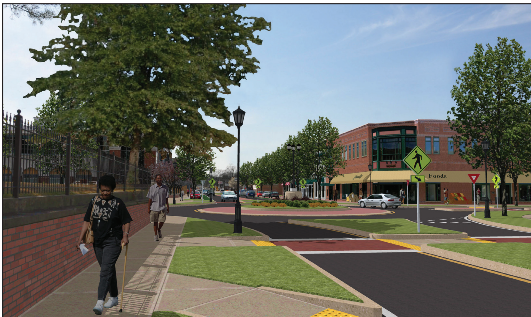
This photo simulation shows a potential improvement, incorporating a round-a-bout, on-street parking, bulb-outs and some minor median installations. The key is showing new development should be placed close to the street, similar to the placement of the 12th Street Mixed-Use Station.
