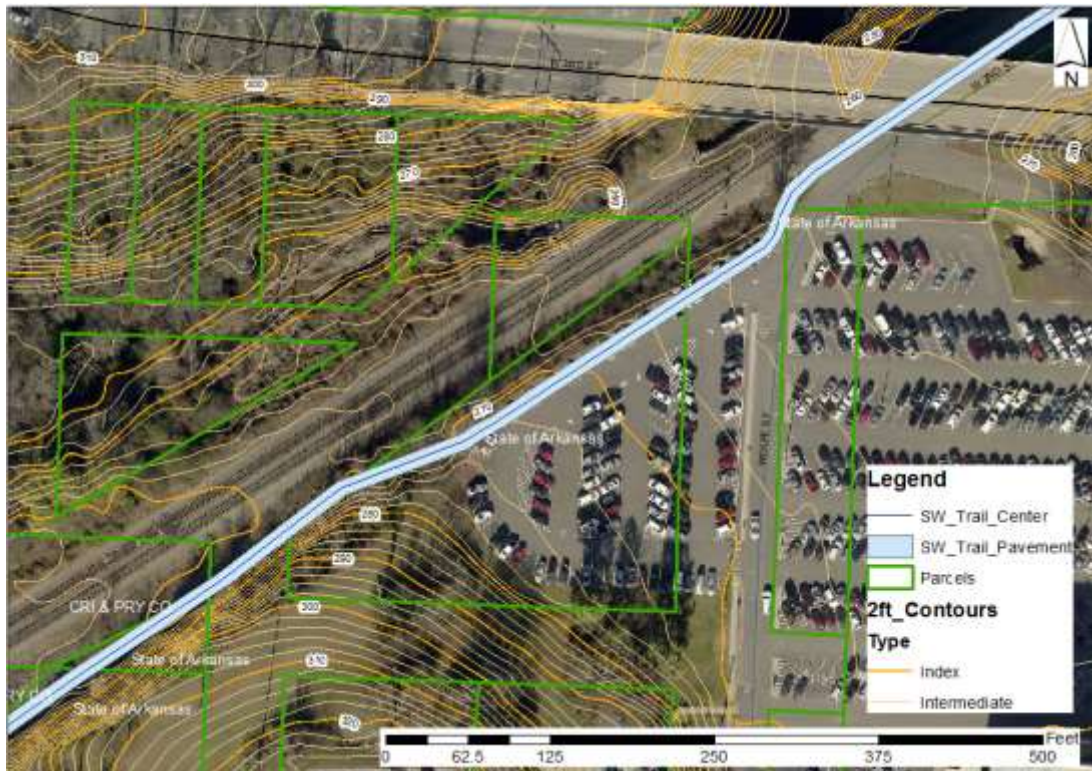
Figure 41. At the State of Arkansas parking lot, we could either run the trail onto the NW-most 18' of a State of Arkansas parking lot (pictured here) or immediately to its NW. If the trail was created in the parking lot, a physical barrier would have to separate parking lot traffic from the trail and a row of parking would be lost. If the trail were created NW of the parking lot, the slope would likely require a retaining wall (expensive). The closest setback is 24', just south of 3 rd St.; creating a trail just NW of the parking lot would not bring the trail setback closer to 24'.
