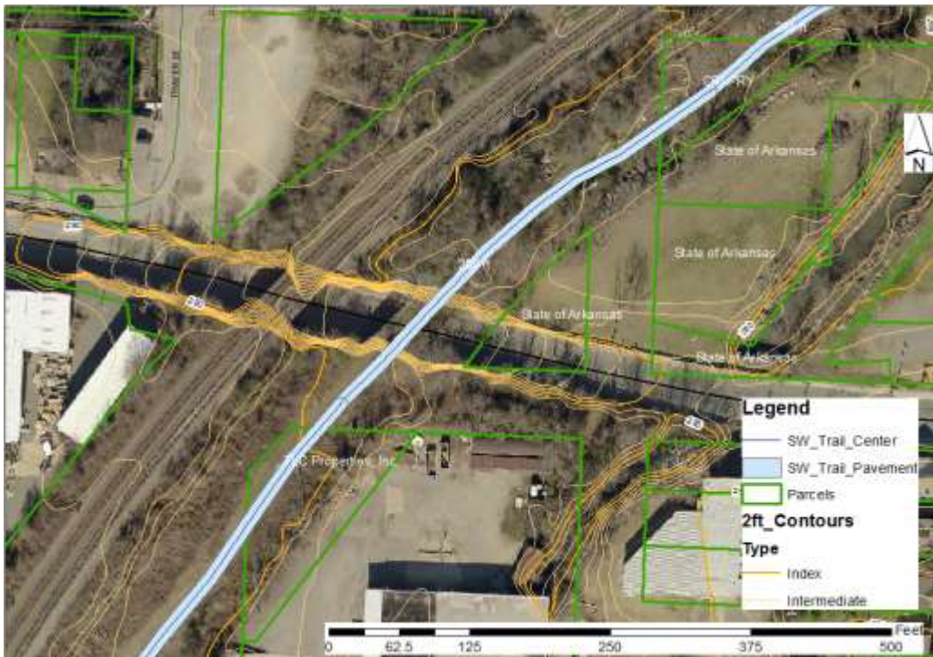
Figure 45. The trail may cross within CRI & PRY CO and TLC Properties. The closest setback is 79'. The trail crosses 7 th St. via an abandoned U.P. bridge.
