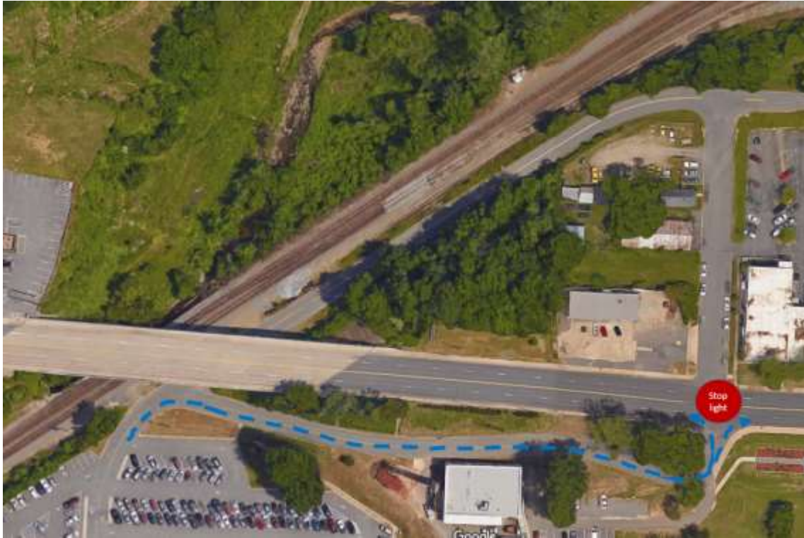
Figure 38. Eliminate vehicular traffic on 2 nd St. Yet another option would be to eliminate vehicular traffic from 2 nd St. entirely and increase the utility of the blue arrow access road for vehicles coming from and getting onto 3 rd St. by adding a traffic light at this intersection. Care would have to be taken to time the light with the traffic light at 3 rd and Martin Luther King to the right of the picture to avoid traffic issues on 3 rd St.
