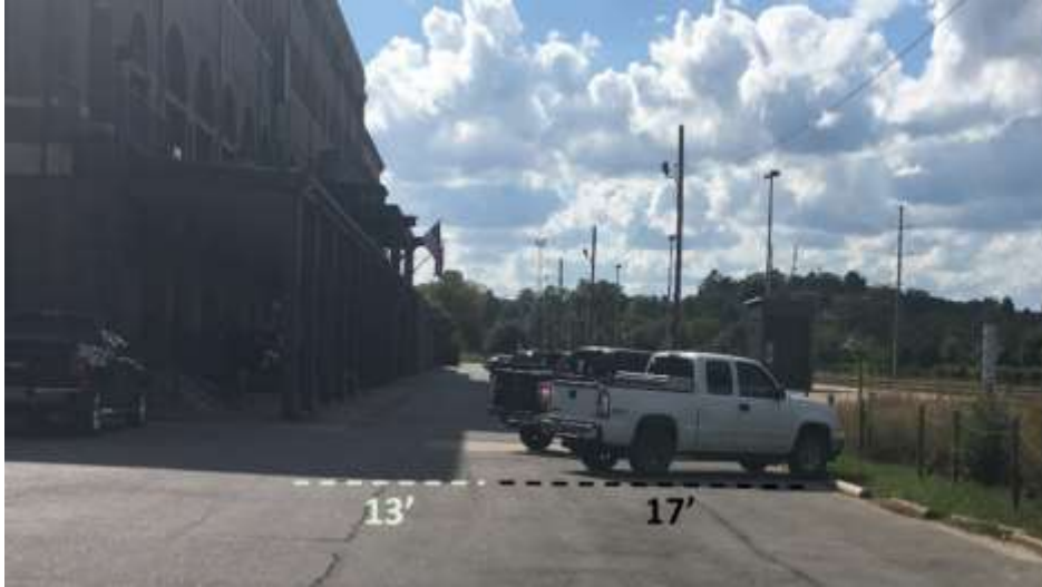
Figure 15. This is the space behind Union Station as it is currently. The distance from the building to the end of the pavement is 30', 17' for parking and 13' for drivethrough. There is ~20' of space north of the parking lot and south of the platform fence, but a slope, ramps with handrails, lightpoles, and the building in the center-right of this Figure make a trail unlikely there. The Corridor could not safely share this space with vehicles. Vehicles pulling out of their parking spaces would be pulling into the 13' drivethrough we would call the "Corridor", a car parked between trucks would be backing out blindly. The minimum standard for the Corridor is 18' of ROW; this drivethrough does not meet this standard. Imagining this area as a bicycle and pedestrian-only space, the area of highest pedestrian traffic, on the eastern end and center of the building, includes a pedestrian canopy. Pedestrians coming from the building and trail users would have lines of sight to see one another. Landscaping could make this area a destination.
