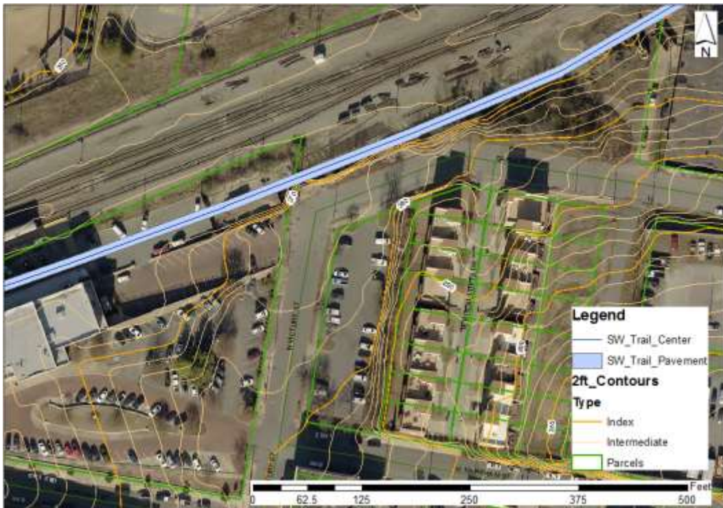
Figure 14 – Union Station BikePed Zone Option. Corridor Route from LaHarpe to the train station. Circumventing the train station is a challenge. One option would be to create a pedestrian and bicycle space (vehicle-free) behind Union Station. The trail run close enough to the building to avoid the handicapped access ramps to the train platform. The closest setback is 54'.
