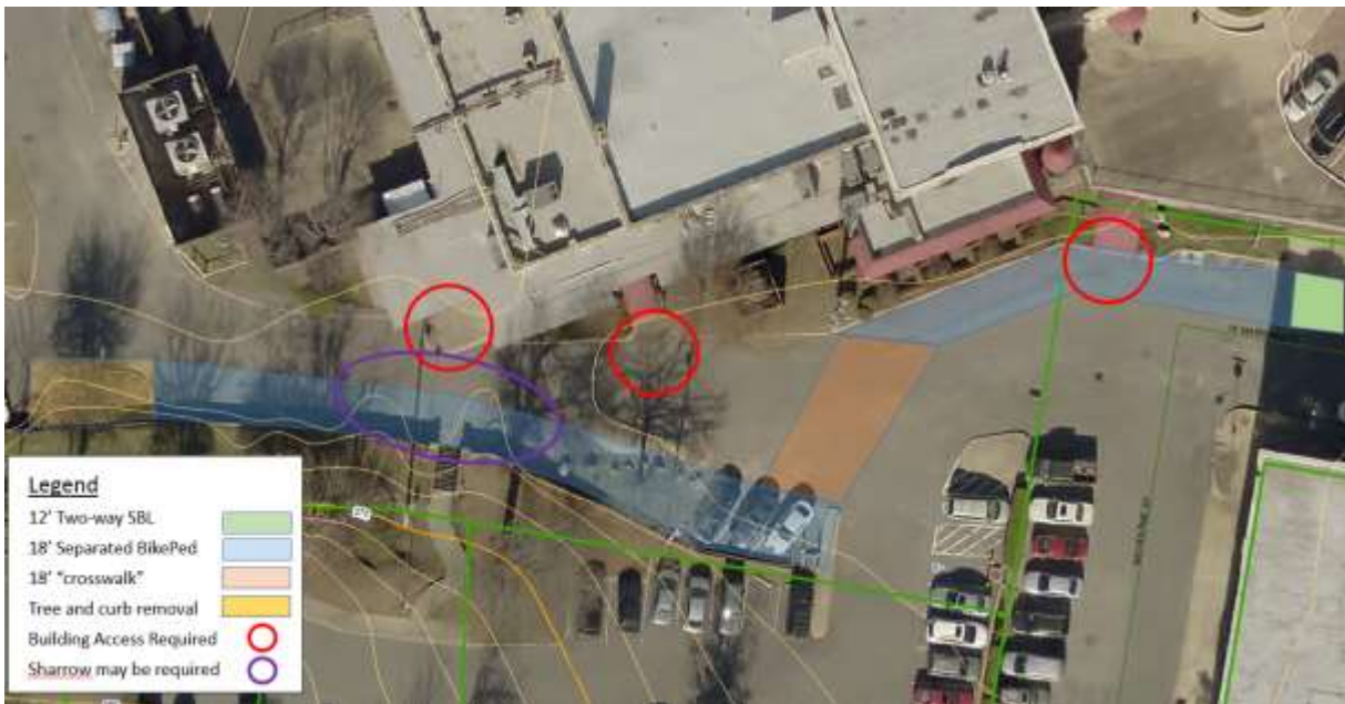
Figure 30. Close-up of intersection of W. Markham and Woodlane. Balancing the needs of the Corridor with vehicular traffic and building access in this area is problematic. From right to left, at the end of W. Markham’s sidewalk, the two-way SBL will convert to a separated BikePed trail. Physical separation must break at the building entrances (red circles). Three parking spaces may need to be removed immediately south of the crosswalk, and the area within the purple circle may have to be a sharrow due to the width between the building and the stairs. Mark Webre suggested we may be able to move the stairs south to create better separation between the Corridor and vehicular traffic. Removal of the tree and curb in the yellow area could allow some parking just off the figure to the left to be retained.
