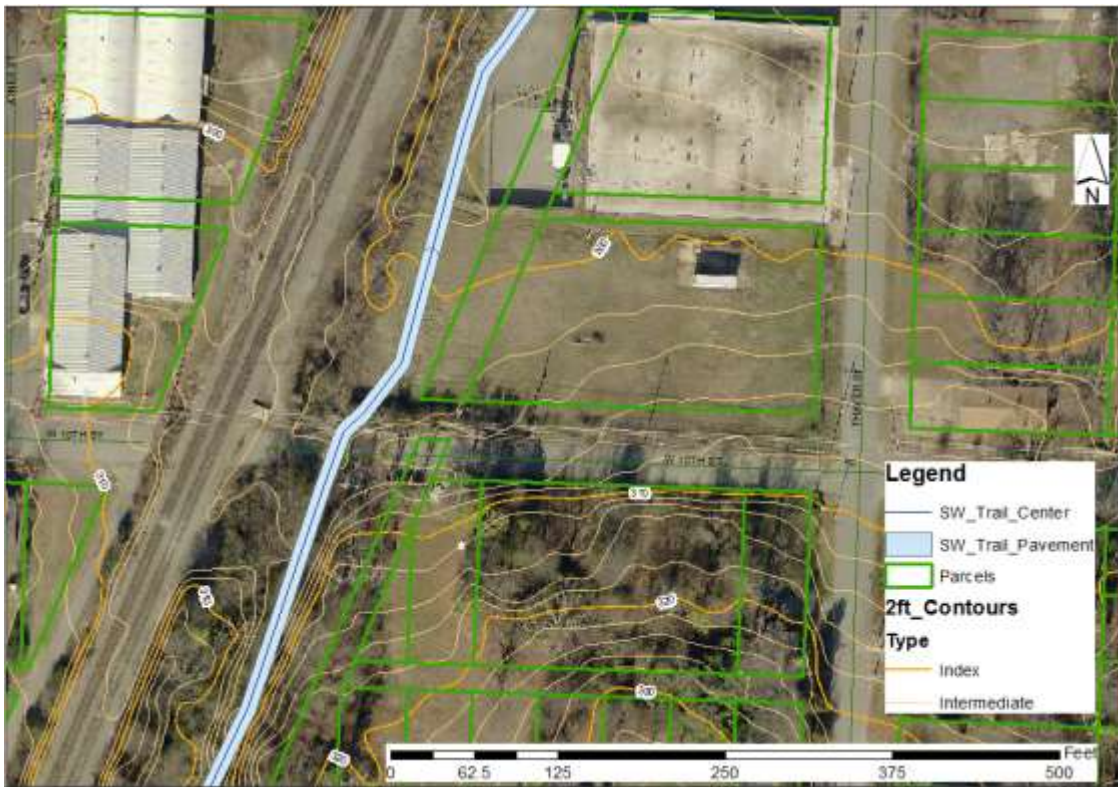
Figure 47. Note the berm starting just south of 10 th St. separating the trail route from active track. The closest setback is 69' in this figure.
