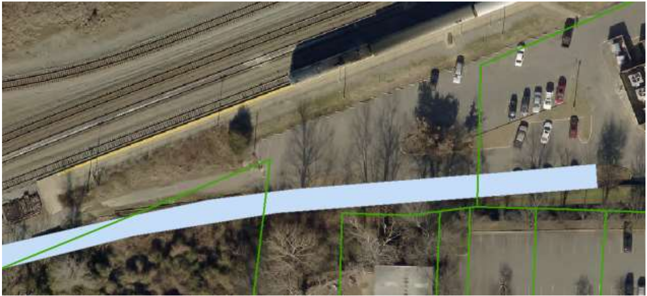
Figure 31. Creating an 18' ROW (blue bar) with physical separation would remove the parking along the south wall, but vehicles would still be able to circumnavigate the parking lot island (especially if one-way counterclockwise traffic arrows were installed). If parking capacity is a concern, the parking island could be removed to create additional parking.
