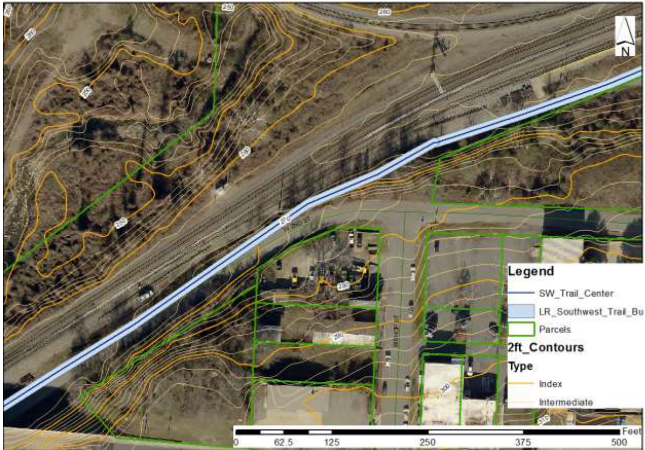
Figure 33. The BikePed Zone behind Union Station and the Victory/Markham Street options both converge approximately at the right edge of this figure. At that point, the Corridor is approximately at 262 ft. above sea level. From right to left, the Corridor will have to go upslope to meet 2 nd St. (which is itself descending at and after its turn southwest). The Corridor will not run on what is now 2 nd St. at its turn southwest (at 276 ft. above sea level), but will instead briefly run on the slope alongside it so that the Corridor is never higher than 270 ft. above sea level. After clearing Curry’s property (the property immediately south of 2 nd St. when it turns southwest), the Corridor will run on what is now 2 nd St. 2 nd St. could either be recreated to the southeast of where it runs now, could be limited to one vehicular lane, or vehicular traffic could be removed from it entirely.
