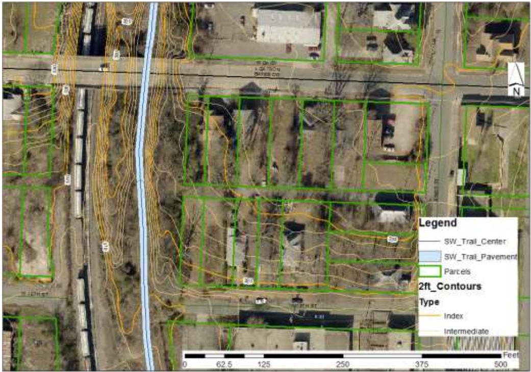
Figure 51. The trail continues to follow the valley of the abandoned UP line and cross Daisy Bates Dr. Note that the berm ends just north of 15 th St. The closest setback is 78’ in this figure.
