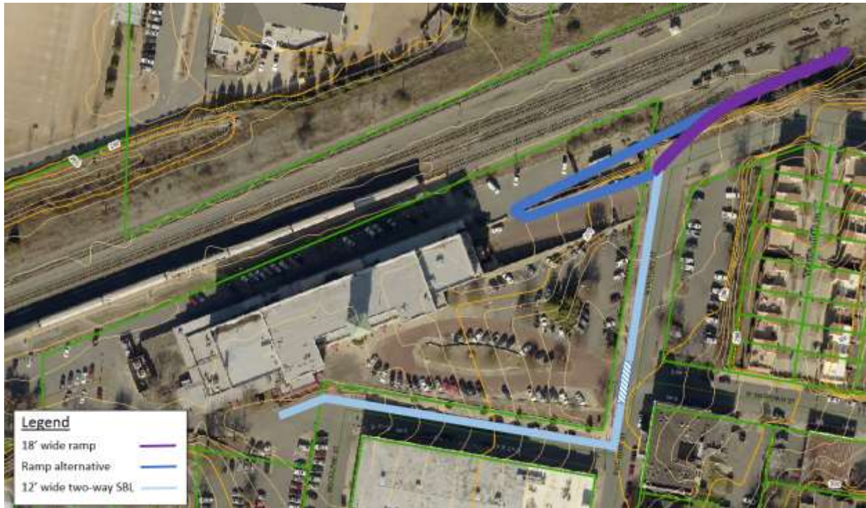
Figure 21 - N. Victory St./W. Markham St. Connection Part 1. Either we would build a ramp to N. Victory St. (about a 10' elevation change, see contours) or route an 18' ROW up the existing brick ramp. Using the brick ramp would be problematic: 1) neither the 180° turn required at the entrance of the brick ramp nor the 120° turn required at the top of the brick ramp would meet Corridor standards, 2) either we would close the bottom of the brick ramp for vehicular traffic or risk BikePed vs. vehicle problems in bind turns (see also Fig. 15), and 3) 13 parking spots would be removed on the brick ramp.
