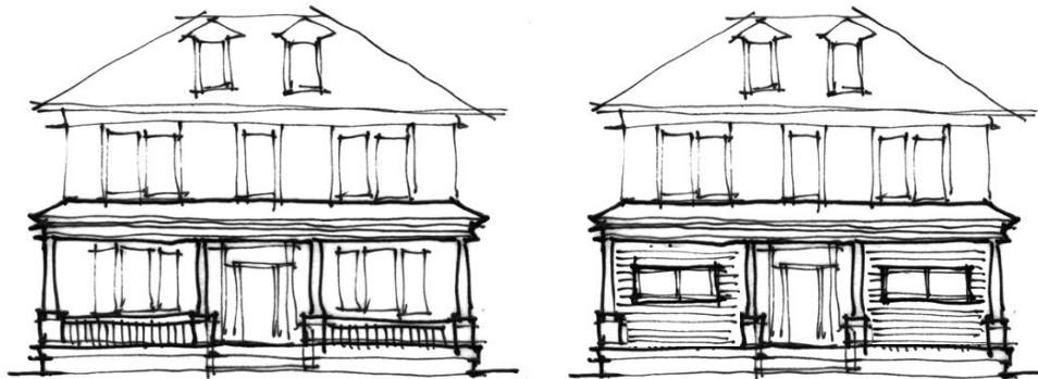
Figure 21. Left, Appropriate porch style. Right, Inappropriate example of filled in porch
