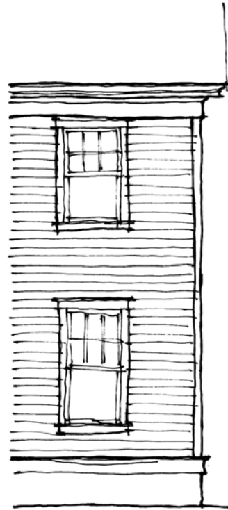
Figure 24. Detail of siding showing all appropriate trim pieces for styles prior to Modern.
