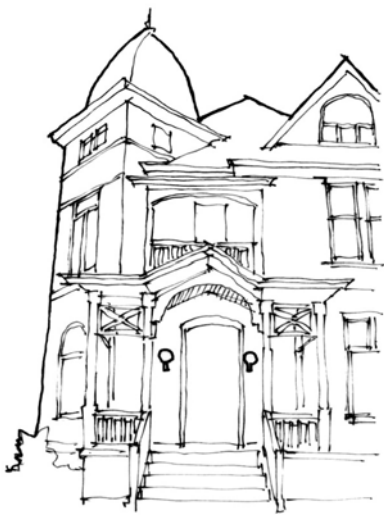
Figure 57. Proper placement of sconces at entry.
