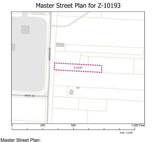
Jamison Rd is a Local Street on the Master Street Plan. Local Streets are roads designed to provide access to adjacent property with the movement of traffic being a secondary purpose. The standard Right-of-way is 50'. Sidewalks are required on one side. This street may require dedication of right-of-way and may require street improvements.
