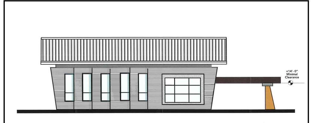
.....view looking to the northeast as passing by John Barrow Road (opposite side, same). One story stab on grade (all ADA accessible) with steel framed superstructure clad with brick masonry; EIFIS wall cladding and gable shaped / metal paneled roof finish......
