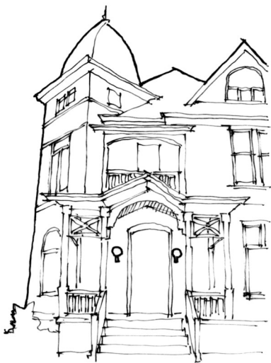
Figure 57. Proper placement of sconces at entry.
