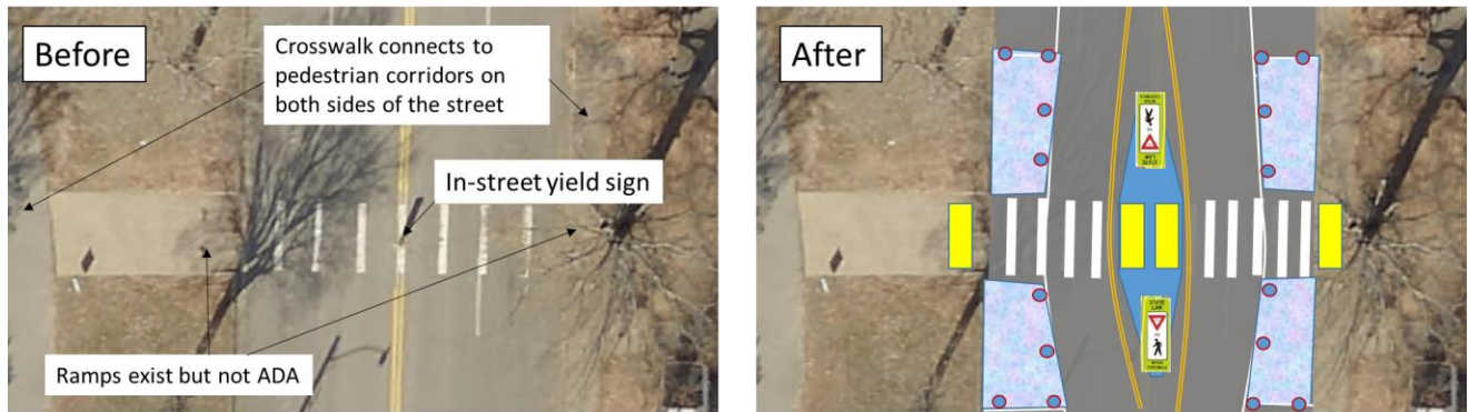
Figure 8. Crosswalk 1 (Fig. 2) has existing pedestrian infrastructure on both sides and existing ramps. I propose to: 1.1 install road diet Monroe (no resurfacing necessary because lane geometry remains the same), 1.2 keep hi-vis crosswalk markings, 1.3 install pedestrian-scale crosswalk lighting, 1.5 keep in-street crosswalk signage, 1.6 install “curb extensions” with removable bollards and street art, 1.7 install pedestrian refuge island. Because ramps currently exist, we could forgo the raised crosswalk (1.4).
