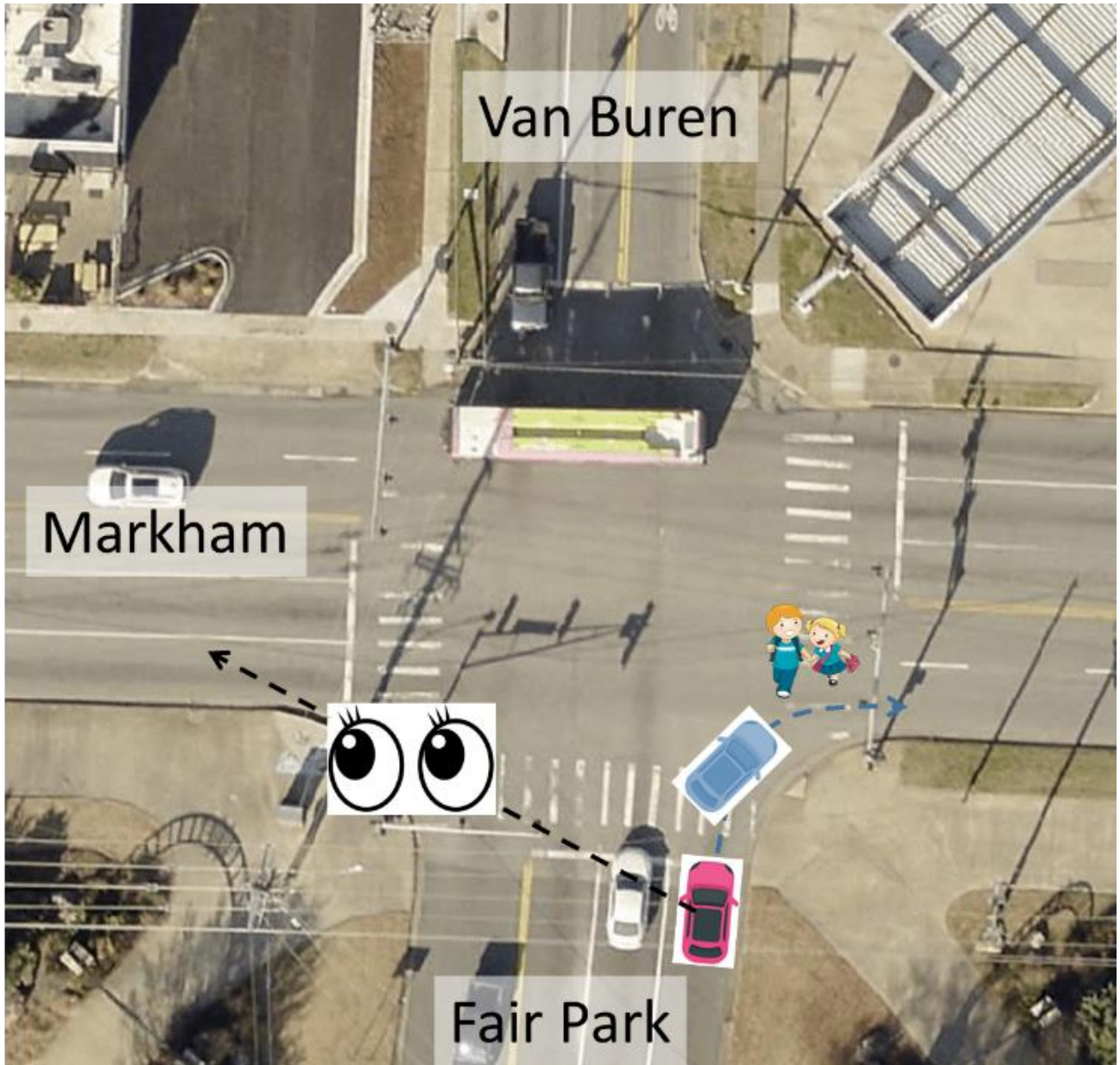
Figure 16. When a controlled intersection has no right-on-red restriction, the driver seeking to turn right on red is waiting for a break in traffic to quickly accelerate into the turn. Her eyes are looking away from the conflicting crosswalks in front of her and crossing the street she's entering in order to time her turn. This pattern is a common cause of car vs. pedestrian collisions at intersections. If the City were to route the Jonesboro Children's Trail to this intersection, it should at the very least not allow right turns on red.
