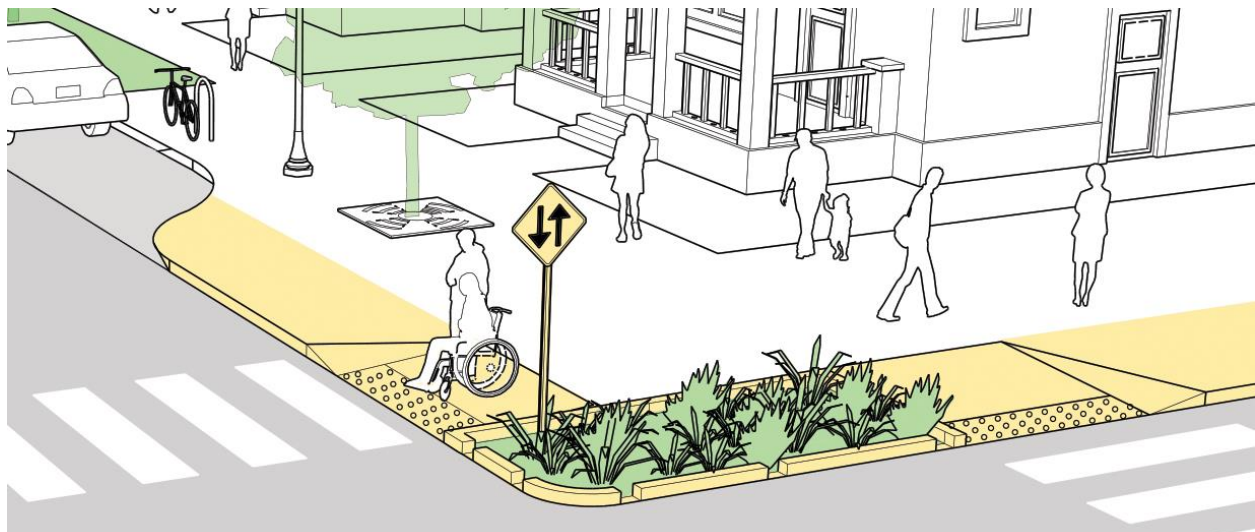
Figure 7. Curb extensions decrease turning radii (calming traffic), create more awareness of pedestrians, physically prevent cars from parking too close to the crosswalk, and limit the exposure of pedestrians to vehicular traffic. Curb Extensions , Urban Street Design Guide, NACTO
