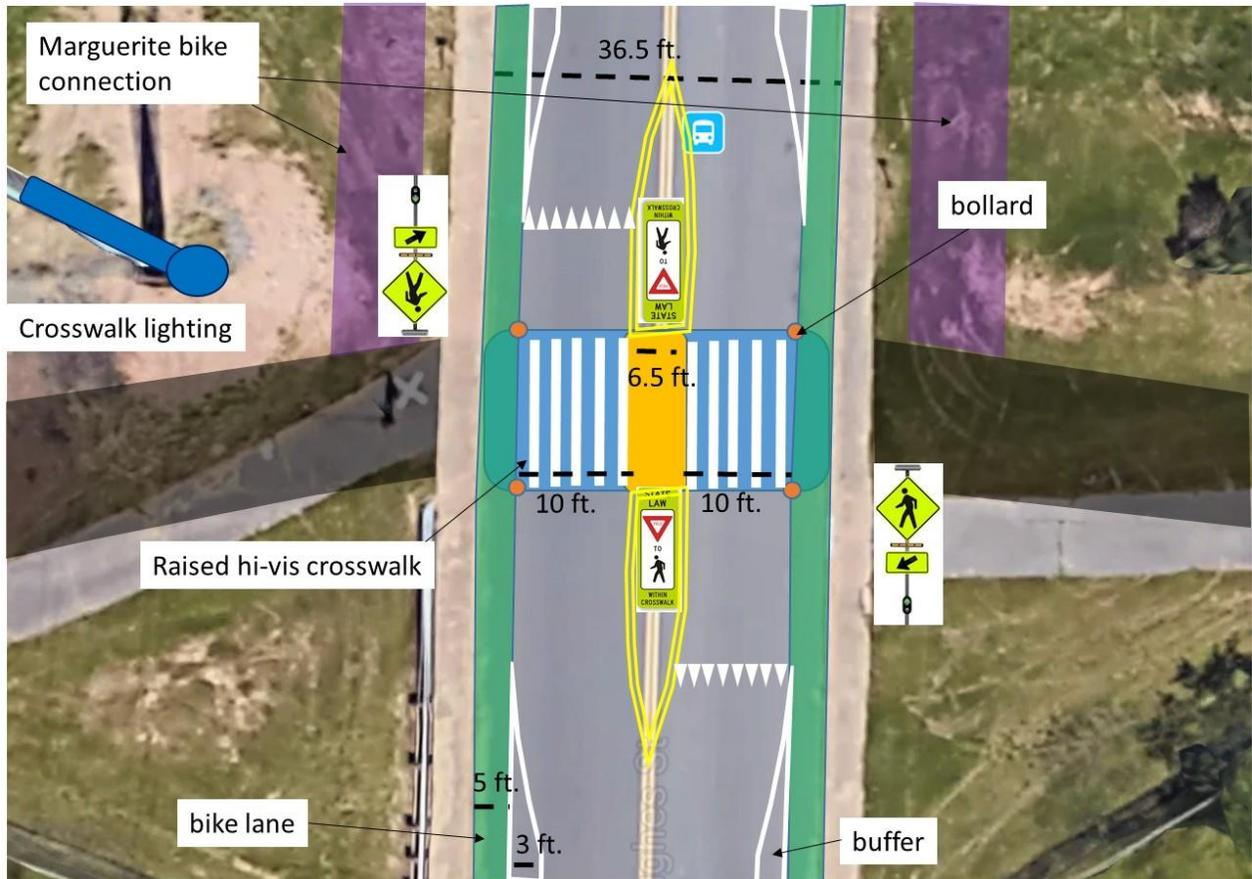
**Figure 8.** Acknowledging that trail alignment encourages trail users to cross here, crosswalk countermeasures could make this crossing safer, but likely not safe enough because of severe limits to sight triangles (Fig. 8).
